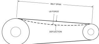
Fig. 37 — Fan Belt Tension
